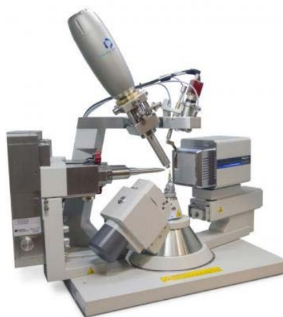
Rigaku XtaLAB Synergy-S X-ray diffractometer for single crystal X-ray diffraction
