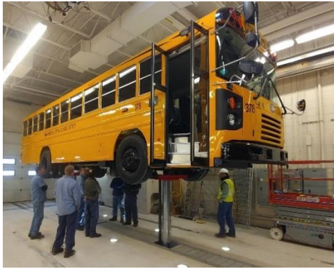
Complete access to the vehicle enables safe and efficient service and maintenance. Here, maintenance workers inspect a school bus on Stertil-Koni's high-pressure telescopic piston lift, the DIAMONDLIFT
