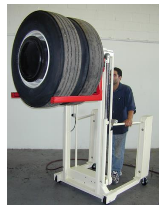
A high lift wheel dolly provides safe, ergonomic removal of vehicle wheels. That's key because two commercial wheels, complete with drums, could weight up to 1,000 lbs.
