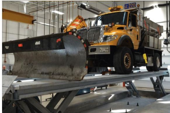
Platform lifts are designed for rapid drive-on, drive-off maintenance. Here, the Stertil-Koni Skylift Washbay model with a water-resistant stainless steel construction proves ideal for undercarriage cleaning, reducing grime built-up around engines.
