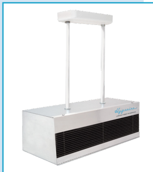
Figure 2 - Shows the top of Hygeaire® Model LIND24-EVO-2PM (above). Note the two mounting holes on the top of this fixture (these are for the Pendant Mount Canopy Set attachment). The fixture is to be mounted at a minimum height of 7 feet from the bottom of the fixture to the floor, in a location that must be able to safely support 32 pounds.
