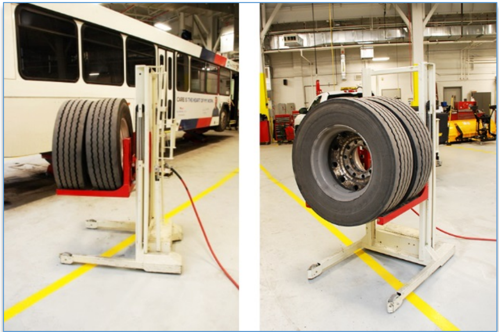
Wheel dollies are ideal for installing and removing the wheels on raised buses and trucks
