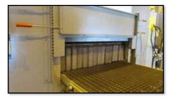
preheating conveyor oven has a maximum temp of  $1,000^{\circ}$  F with guaranteed temperature uniformity of  $\pm 10^{\circ}$  F at 950° F
