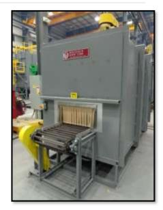
attachments was utilized to transport the product through the system and a variable frequency drive provides adjustable speed control. Fabric ribbon curtains are located at both ends of the conveyor to prevent heat spill out.
