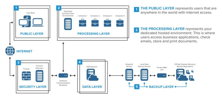
THE SECURITY LAYER represents the corporate security infrastructure designed to protect you from malicious viruses, spyware, and hackers. THE DATA LAYER represents the subsystem of the IO environment that stores all of your company's data. **THE BACKUP LAYER** represents the subsystem of the IO environment that stores & backs up all of your company's data.
