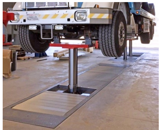
In 2018, Stertil-Koni enhanced its inground piston-style DIAMONDLIFT with a continuous recess system – a first in North America
