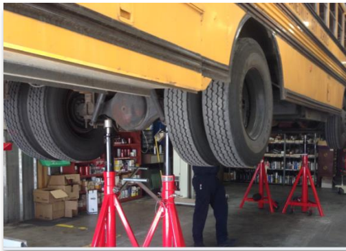
Stertil-Koni support stands are available in capacities from 7 to 18 tons per stand
