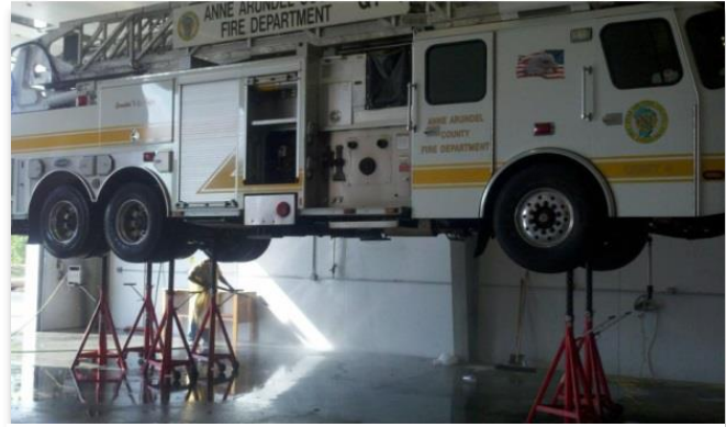
Support stands can be adjusted to the desired height to support the vehicle. Several Stertil-Koni models allow six-inches of fine adjustment via an ACME screw
