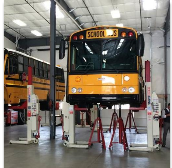
Support stands have become an indispensable and reliable piece of shop equipment for service and repairs
