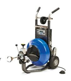
The limit can be set high for large drains or low for sink lines. Operators can also select how tension is released: quickly with little resistance, or slowly with more resistance.
