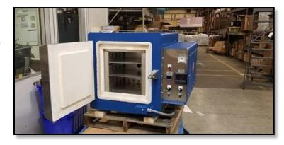
long life and reliability. Both are ideal for tool room, plant maintenance, and production applications that require maximum heat-treating, hardening, and tempering capabilities in a minimum amount of space.
