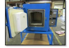
The box furnaces have work chamber dimensions of 12" wide x 18" deep x 12" high. The Temperite™ and Treet-
