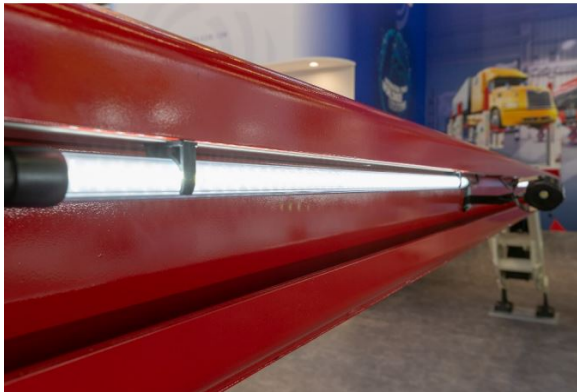
New high-performance Stertil-Koni LED lighting tubes on the company's true vertical rise platform lift, the SKYLIFT
