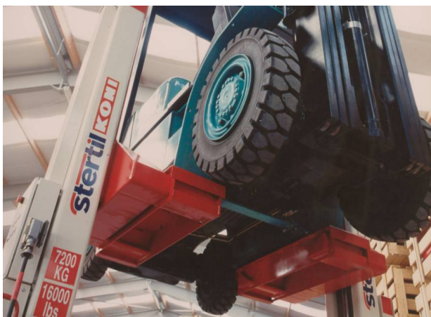
Stertil-Koni forklift adapter kits make servicing a safe and easy option for technicians while affording wheels-free lifting
