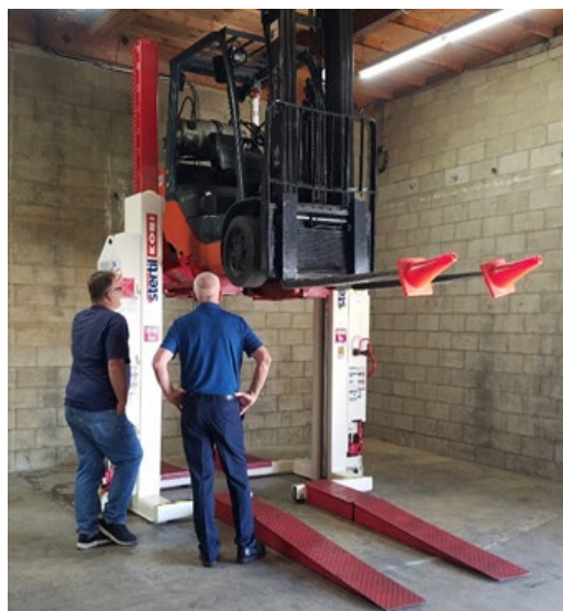
Stertil-Koni recommends modular drive-on ramps for safe and time-saving maintenance
