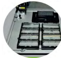
Instrument iTWO™ - equipped with a source MTP or vial holder, wash station, droplet volume detection system, head camera for QC, flexible deck configurations, where MTPs, glass-slides and vial can be placed next to each other.
