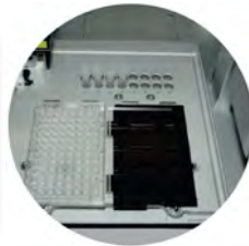
Instrument iTWO™ - equipped with a source MTP or vial holder, wash station, droplet volume detection system, head camera for QC, flexible deck configurations, where MTPs, glass-slides and vial can be placed next to each other.
