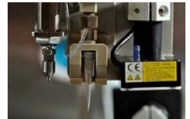
M2MD for 10+ nL dispensing with a disposable tip
