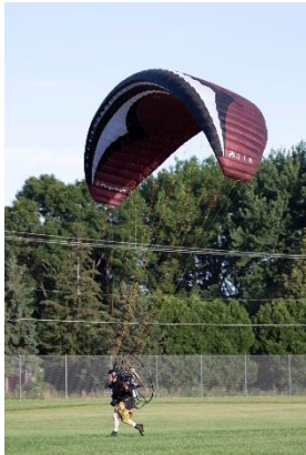
Figure 1 Powered paragliders, like other ultralights, fly at low altitude and can operate from small fields
