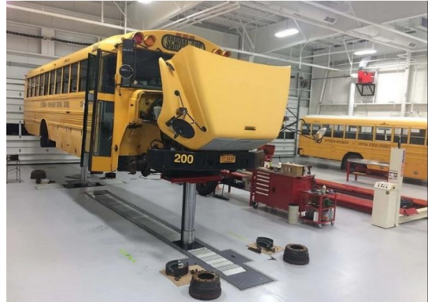
Wheel-free lifting via a high-performance, telescopic inground piston lift are hallmarks of the Stertil-Koni DIAMONDLIFT
