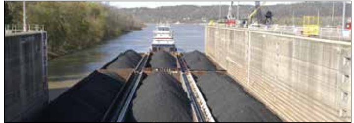
A six barge tow tied off on the downstream side of Markland Lock & Dam's 600-foot lock on the Ohio River, 531.5 river miles below Pittsburgh. Towboats push up to 15 barges when navigating the inland waterway system, but a lock can accommodate only six to nine barges at a time. One barge has the capacity to safely transport 1,500 tons of products (photograph: Army Corps, November 2009).
