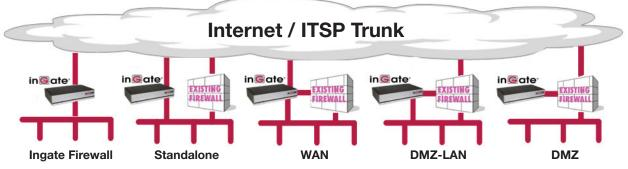
QoS (voice quality over data-crowded accesses) is provided by the SIParator. DMZ-LAN & DMZ modes also require QoS setup in existing firewall.
