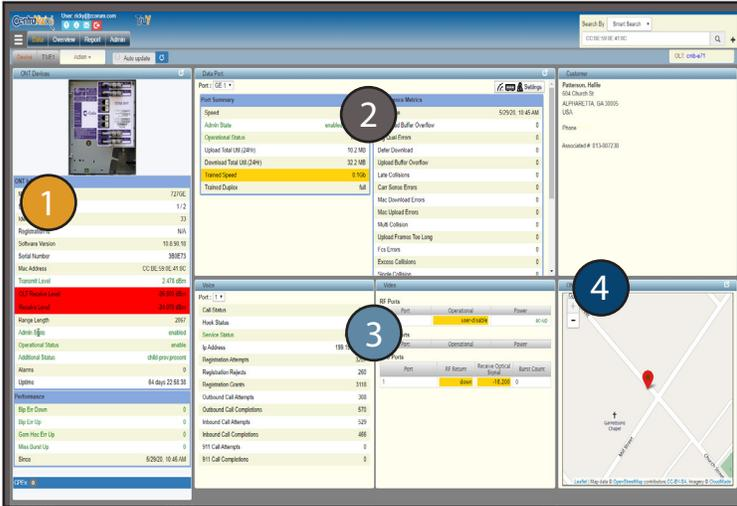
See optical levels, errors (BIP, GEM, Burst) and easily see any alarms for the ONT, color coded by alert level. Click to graph this data over time.
