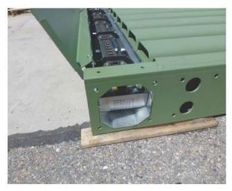
A wedge wire screen, at the fluid discharge end of the Hydropad above ground steel wash pad gutter, filters fine solids that the drag conveyor scraps clean to remove as solid residue. A small above ground sump box and pump connects here to pump collected water to a recycle system or other discharge point.
