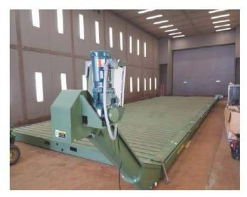
Shown here is the solids discharge lift station where all collected solids are automatically removed from the side gutter. Water separated from solids flow to the opposite end of the Hydropad steel above ground wash pad and are pumped to a either recycling equipment or another discharge point.
