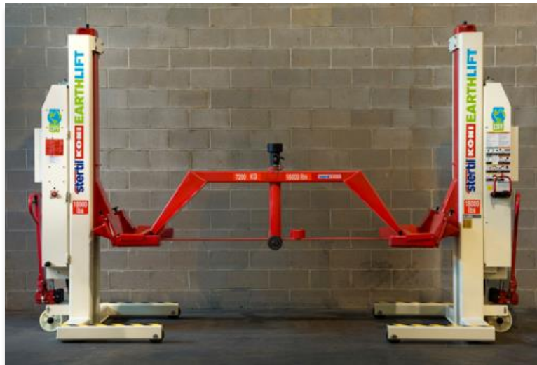
Stertil-Koni Kingpin Cross Beam Adapter, shown here, supported by two mobile Column Lifts
