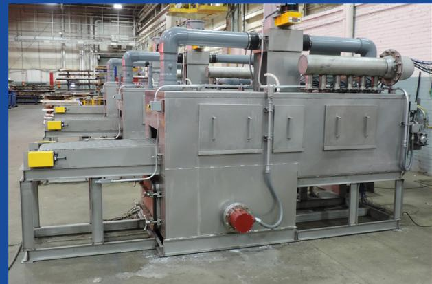
The washer features an inclined conveyor that is 39" at load and 42" at unload.
