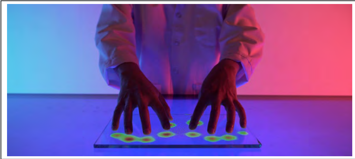
Figure 13: Fully functional 65 inch PEDOT:PSS touch sensor shown in 2020 C-Touch exhibition.
