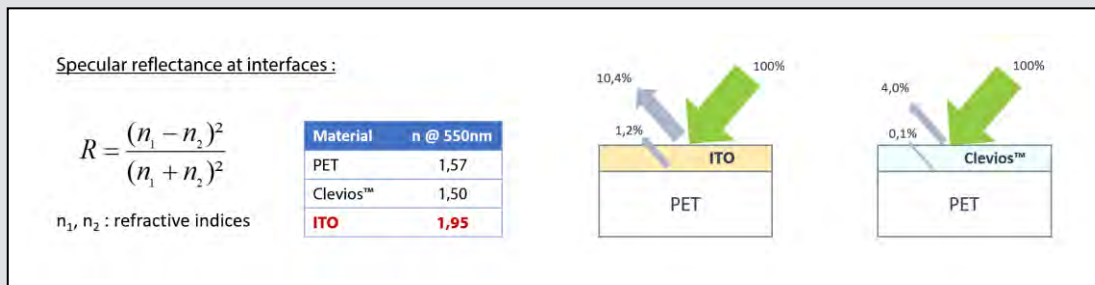
Figure 2: PEDOT:PSS coated PET films exhibit lower light reflection and thus superior optical properties than ITO PET films.
