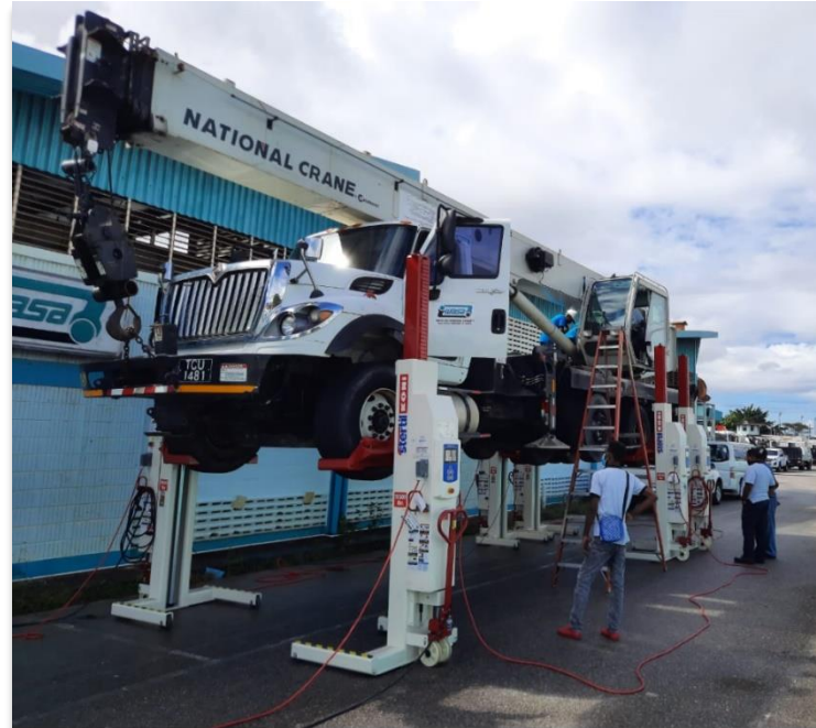
Stertil-Koni Mobile Column Lifts are indeed mobile and can be used outside on a firm, stable surface when wind loads are minimal
