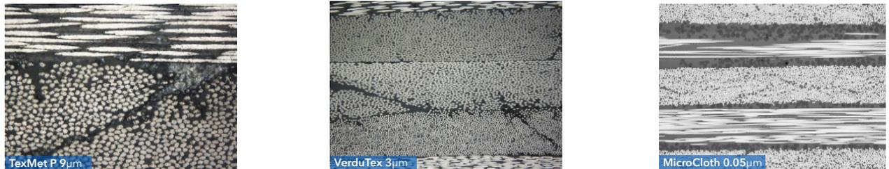
Figure 2 showing surface finish after semi-automatic preparation after 9 $\mu$ m, 3 $\mu$ m and 0.05 $\mu$ m step.
