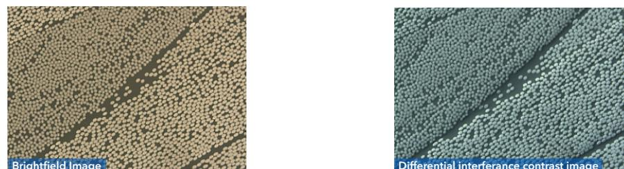
Figure 3 showing surface finish after 0.05 $\mu$ m alumina on Microcloth prepared by manual preparation.
