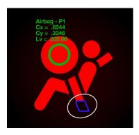
match the exact shape of each illuminated element regardless of component position or orientation. Precise ROI enable VIP to measure the exact brightness, color, and uniformity values of each element or symbol and detect defects within the ROI, identifying issues in substrate etch (ROI shape completeness and integrity), dead LEDs, poorly diffused backlight, and particles within substrate layers.
