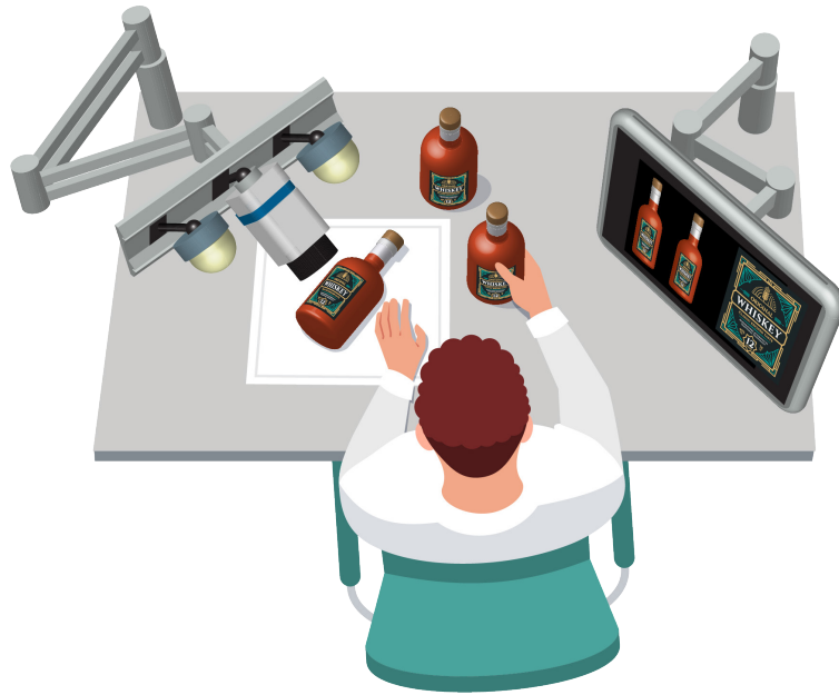
Figure 3: A fully integrated visual inspection system includes a camera, display, edge processing, and pre-packaged common inspection skills, while no code development platforms enable easy customization for unique requirements.
