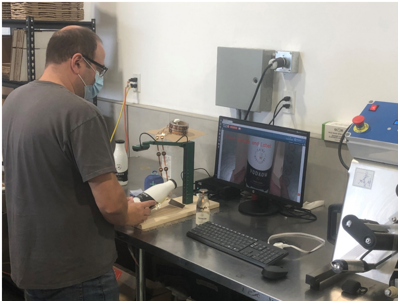
Figure 6: The visual inspection system requires just one "good image" of the bottle to help the operator align labelling.
