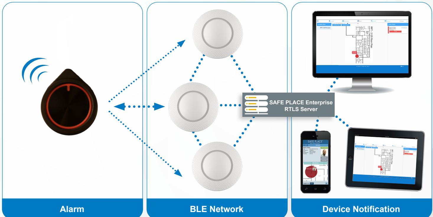
**Rapid response:** When an alarm is activated, location information is collected by the BLE gateway network, then passed through a server to all security-monitoring computers and available mobile devices – all within seconds.
