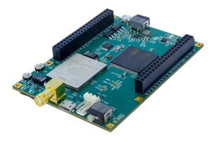
Supports LTE-M, NB-IoT and GNSS
