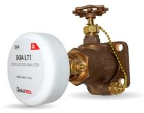
Qualitrol's DGA LT1 is a wireless, self-powered dissolved gas analyzer that monitors hydrogen, moisture and temperature in the dielectric insulating oil. Installation takes minutes because there is no need to install power or communications cables.
