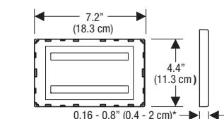
\*NOTE: Customizable surface-even cover plate accepts typical wallcovering materials to disguise the service opening. Minimum finished wall is  $\geq 3/4"$  (1.8 cm) plus cover thickness up to a maximum of 2" (5 cm) total.
